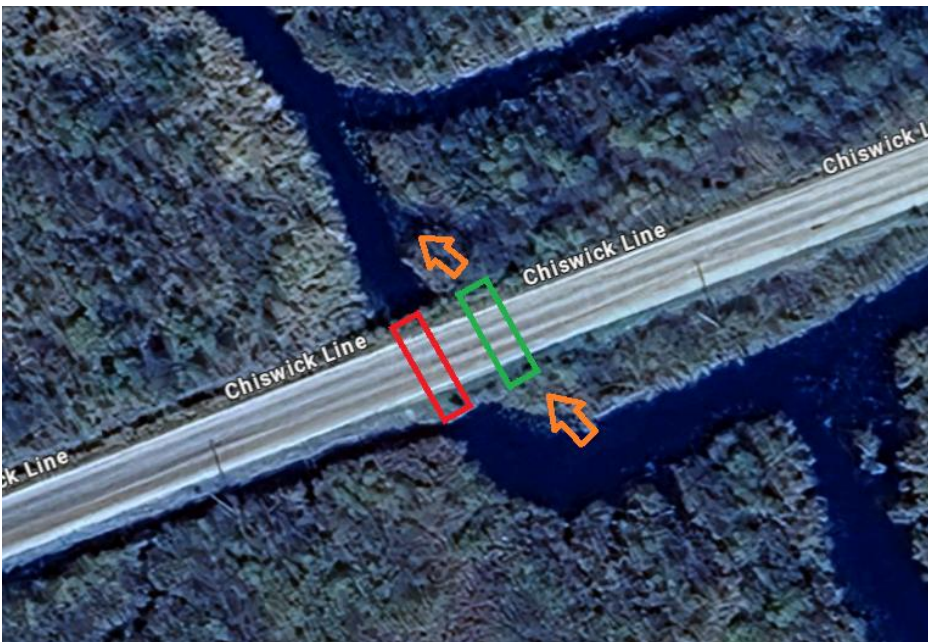
Sketch showing the proposed location of the new multiplate (in green) approximately 30m east of the existing superstructure to be removed upon completion of construction (in red).
